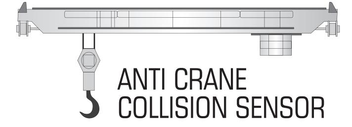
Electronic Switches offers Anti Crane Collision Switch for two over head cranes on the same rail. These units are installed on two cranes on the same rail approaching each other. With these units, the two cranes on the same rail will never collide with each other & thus the damage caused due to collision can be avoided. The minimum distance in between two cranes can be set and will always be maintained. The cranes will be able to move away from each other but not closer.
