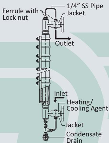
Is employed for heating/cooling of process liquid at temperature other than amb temperature, to prevent its solidification. Heating is done thru` hot water / steam and cooling thru` a refrigerant like freon, propane, or ammonia, which pass internally thru` a SS pipe, gauge chamber to come in direct contact with process liquid.
