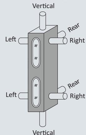
Note : RFG (hook-up & straight thru) and TFG (straight thru) available in above orientations. **TFG (hook-up) not provided in Left x Left and Right x Right orientation.**
